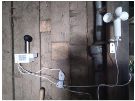
Fig. 2 ► The Pessl and MoBiMets sensors measure humidity and temperature in real time.
